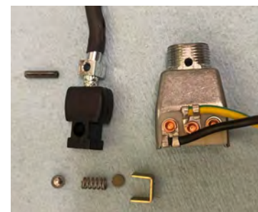
Photo 1 – Disassembled Overdrive switch
