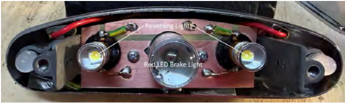
Photo 7 - Modified Reversing Light Completed
