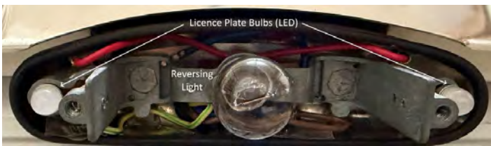
Photo 1 - Internal View of Reversing and License Plate Lights
