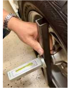
Figure 6 - Measuring the Camber
