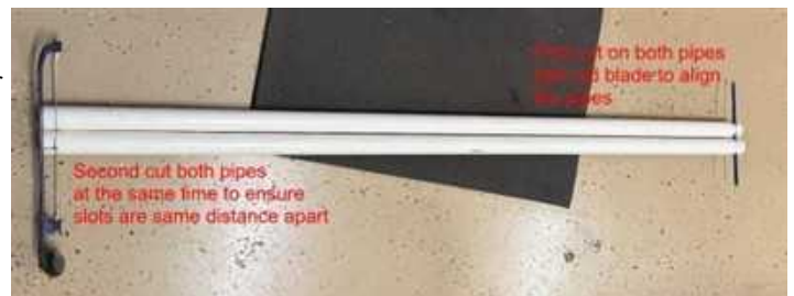
Figure 7 - Preparing the front and rear pipes
