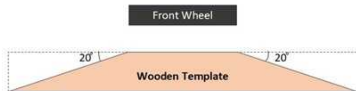
Figure 3 - Castor Alignment Template
